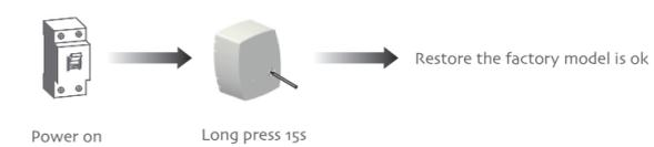
Note: Please use this procedure only when the network primary controller is missing or otherwise inoperable; this operation is Z-Wave part and motor and restore factory Settings.
