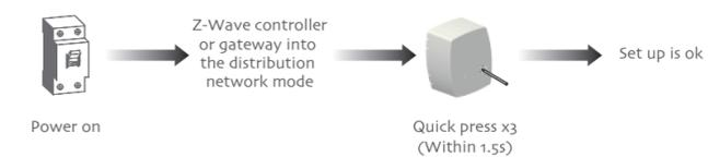
Note: Z-Wave controller or gateway into the mode of distribution network operation reference related operation manual.
