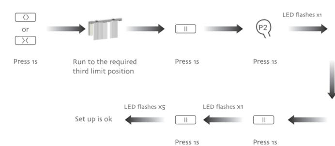
Note: The clear third limit point method same as set the limit point; Long press the stop button for 2s, the motor moves to the third limit position automatically.
